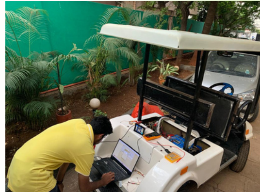
Integration of EV powertrain on golf cart for in-vehicle testing
